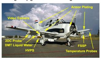
A highly-modified T-28 Trojan used by the South Dakota School of Mines and Technology for storm-chasing and measurement.
