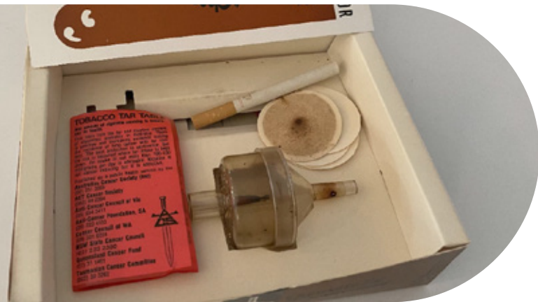
Shane's cigarette tar extractor. The blackened filter paper after "smoking" the cigarette clearly highlighted the health hazard.
