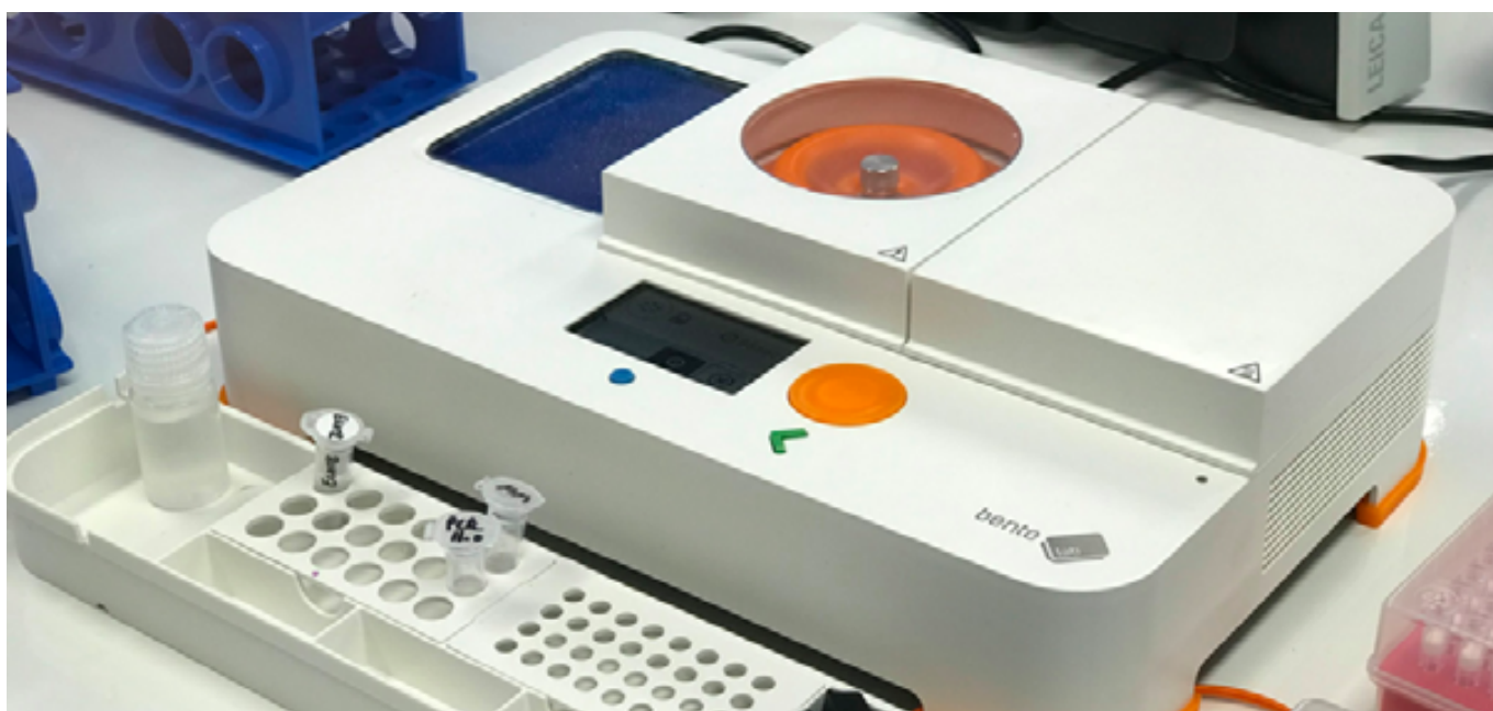
A "Bento Lab". These devices function as a portable molecular biology lab, combining a PCR machine, microcentrifuge, gel electrophoresis, and a transilluminator to amplify and visualise DNA
