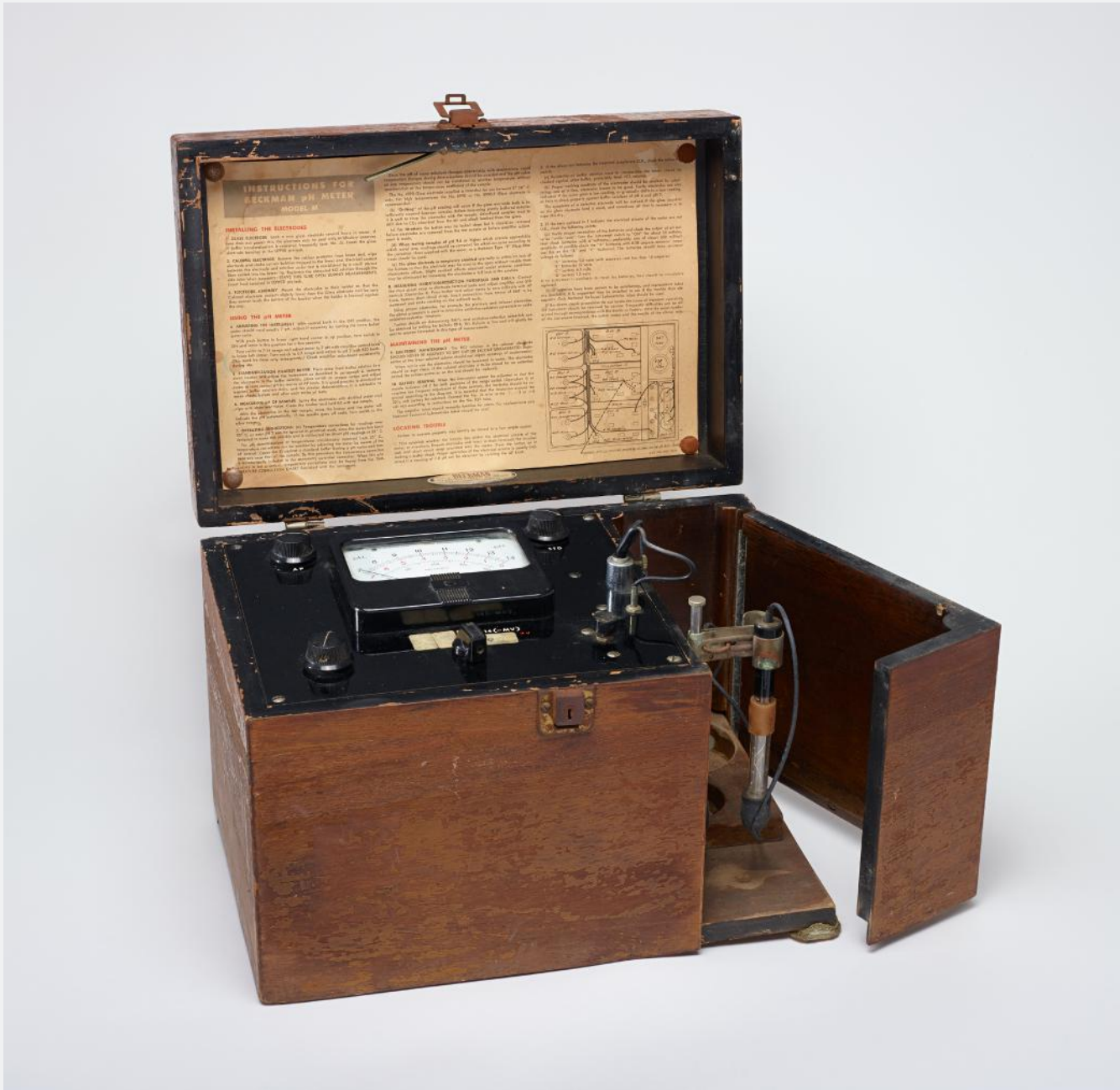
The Beckman Model M pH Meter, first sold in 1937, was the fourth version of Beckman's pH meters to reach the market. Source: Science History Institute (Public Domain).
