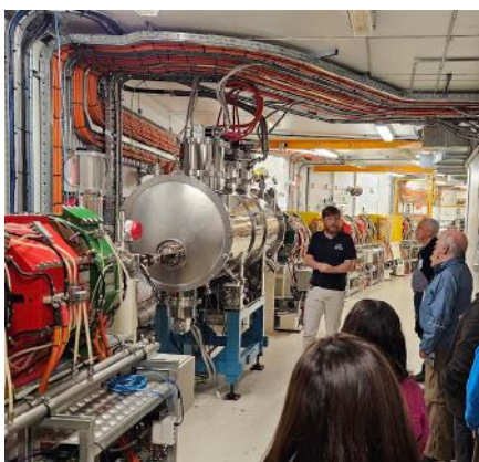
Geographers being shown the huge electro-magnets that bend the beam. Photograph: Ian Rutherford.
