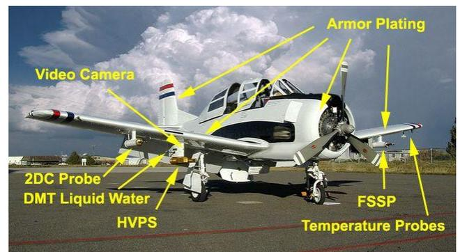
**A highly-modified T-28 Trojan used by the South Dakota School of Mines and Technology for storm-chasing and measurement.**
