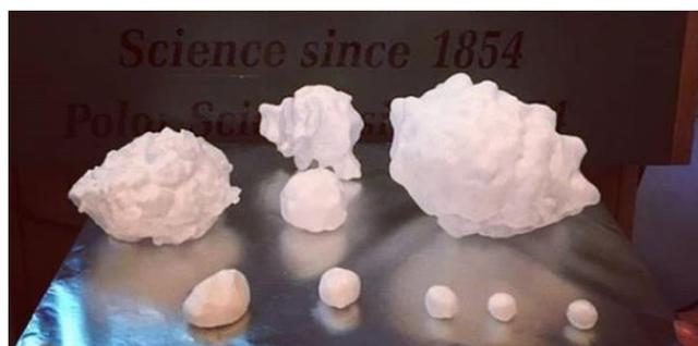
**Dr Soderholm provided physical representations of the range of hailstone sizes, from embryonic to catastrophic! Here they are sitting on a "hail pad," a polystyrene board covered in aluminium foil.**
