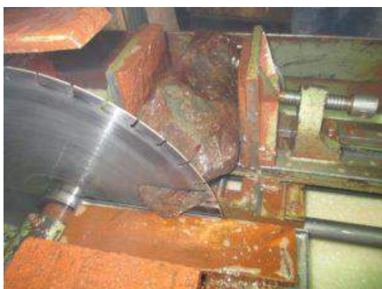
Cutting the Maryborough Meteorite for analysis at Crystal World. Photo: Thomas Kapitany
