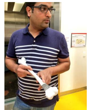
RMIT Biomedical Engineer Dr Darpan Shadid demonstrates how 3D-printed titanium lattice can provide bespoke structural infill for bone, allowing the natural colonisation of the lattice with regenerative bone tissue post-surgery.
